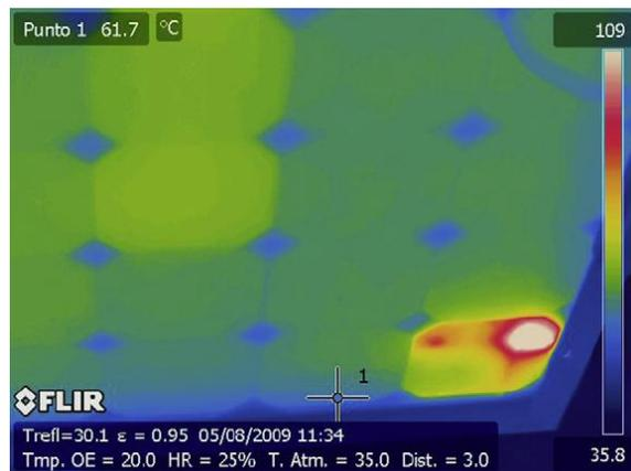
Figure 12: Hot cell in Conventional PV
