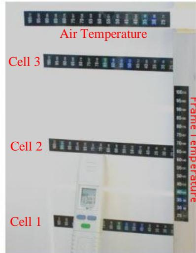
**Standard bypass heats partially shaded cell to 95°C-130°C.**
